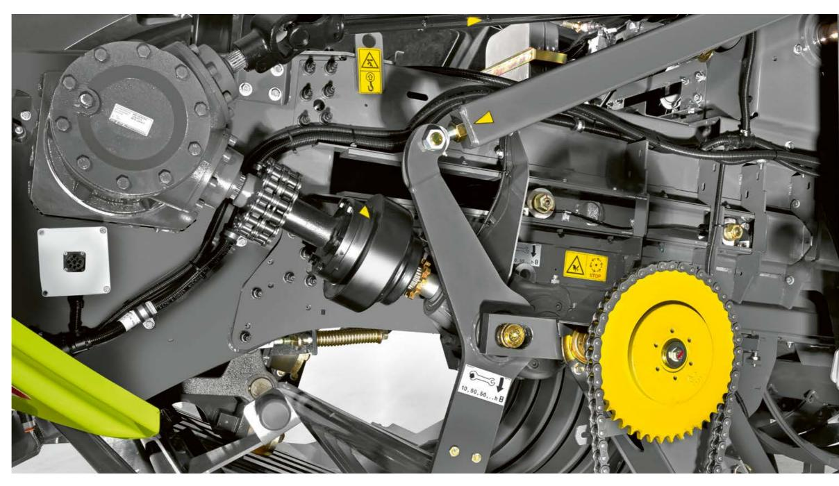
The baling ram is also protected against overload by a safety clutch. All overload clutches automatically reengage after reducing the PTO shaft speed. You'll never need to leave the cab in the event of a blockage. Special protection.
