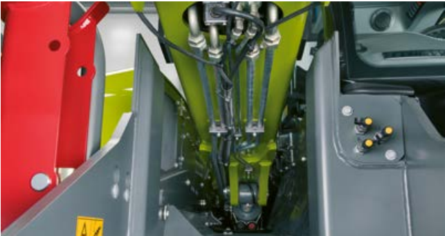
Side telescopic arm guide integrated into the frame as standard with all telehandlers with load capacities above 4,500 kg.
