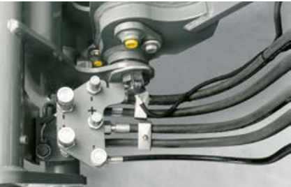
1 Front control circuit 2 Pressure release
