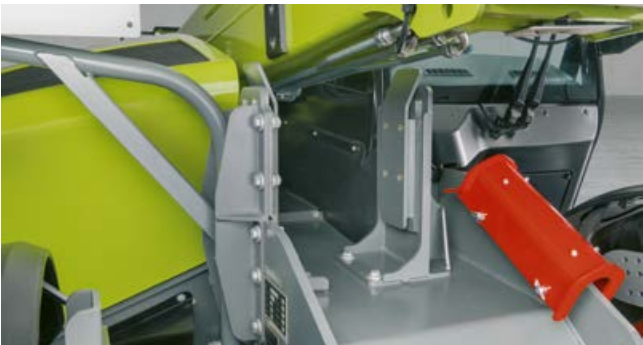
Side telescopic arm guide available for all SCORPION models.
