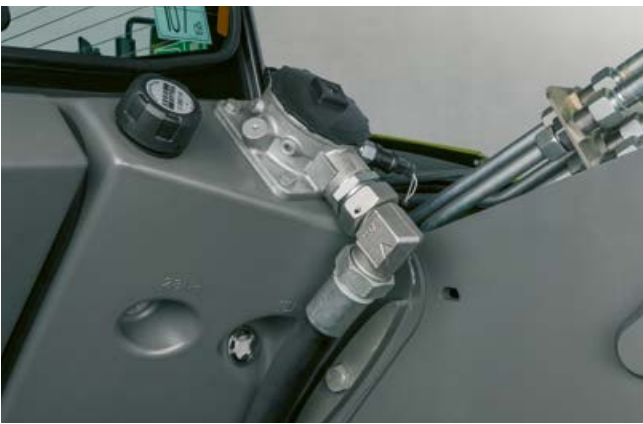
The hydraulic oil level can be conveniently checked via a sight glass. The hydraulic system is protected by a return filter which only needs to be changed after 1,000 operating hours.
