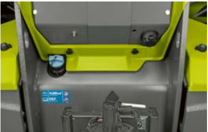
Easily accessible AdBlue®-filler neck filler neck for efficient exhaust gas aftertreatment.
