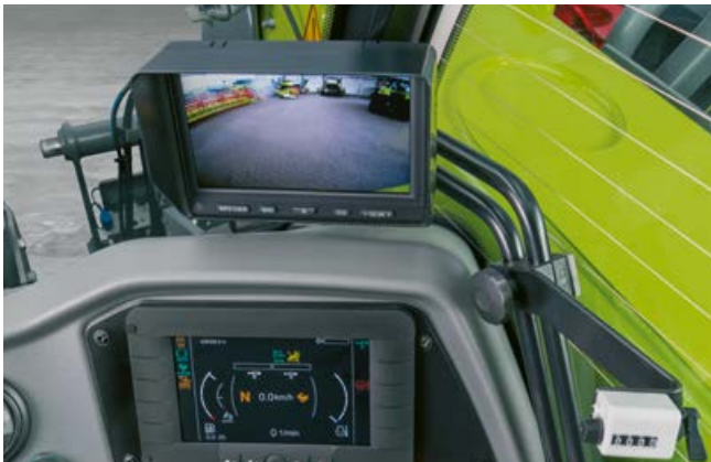
The images from the front and rear cameras are transmitted to the monitor in the cab.
