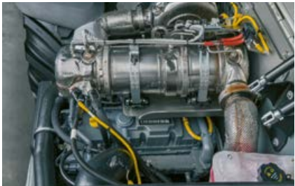
The diesel particulate filter is regenerated automatically.
