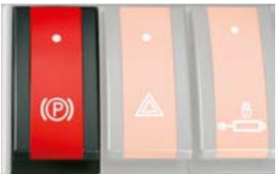
The toggle switch allows the parking brake to be operated manually.
