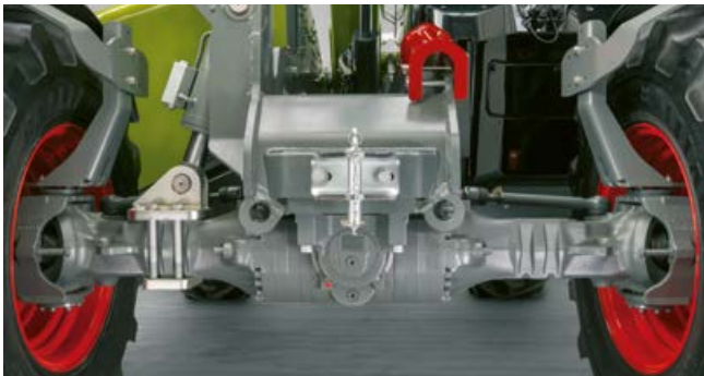
Chassis with hydraulic levelling.
