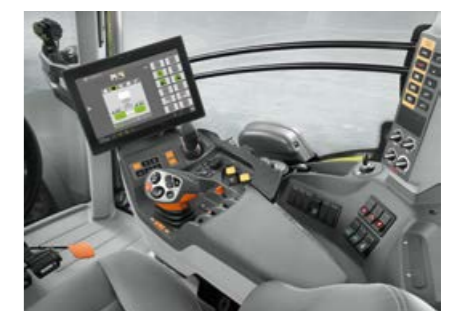
If the tractor is equipped with an ISOBUS-compatible terminal, preselected functions for the CONTOUR can be operated from there
