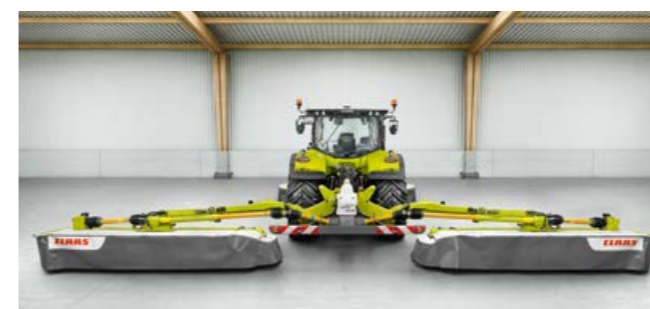
Two hydraulically controllable telescopic arms with continuous adjustment for optimal overlapping in the DISCO 1100 TREND
