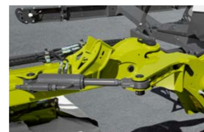
Hydraulic non-stop collision protection – in the event of a collision, the mower pivots up and over the obstacle, and resets itself automatically
