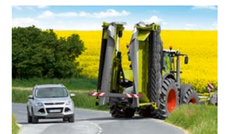
Less than 4.0 m: compact transport position with generous ground clearance in both BUSINESS models
