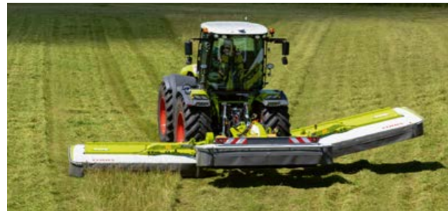
Individual mower unit lift at the headland
